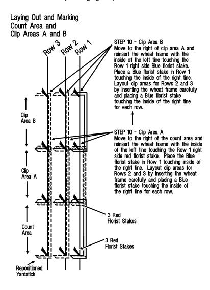
**Step 10:** Laying out and marking Clip Areas A and B.
