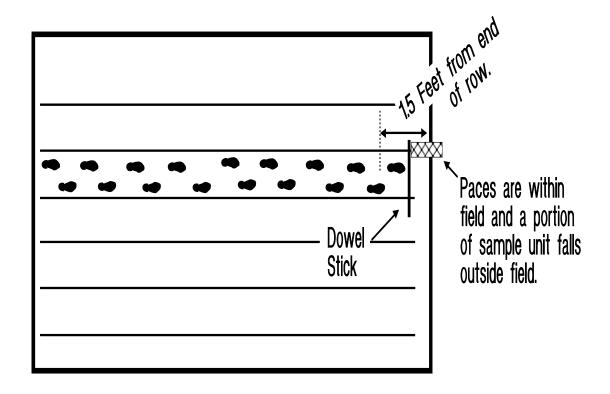
When the number of paces into the field will cause part of the unit to fall outside the field proper, decrease the pace count until the entire unit is included in the main body of the field by 1 1/2 feet.
