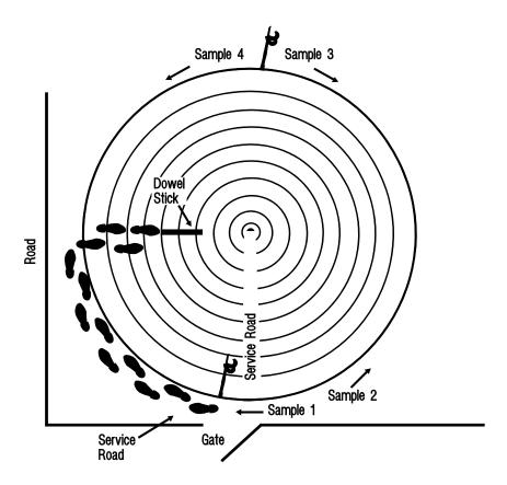
The starting point will be that point first reached when arriving at the field. To locate sample units in a spiral seeded field, use paces as shown on the Form B when walking clockwise along the edge of the field. Then use the number of paces shown on the Form B to count paces into the field. Be sure your diagram on the kit envelope is complete and is easy to follow in locating the sample units in the spiral field.
